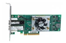
HPE STOREFABRIC SN1000Q 16GB 2-PORT PCIE FIBRE CHANNEL HOST BUS ADAPTER, 699765-001
